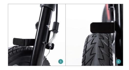
B: If method one doesn't work, please tighten the brake cable.
