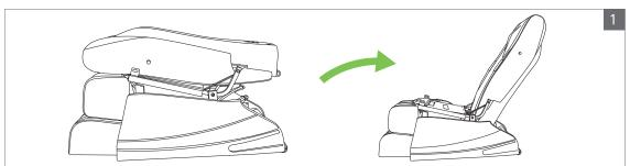
step:1 First, lift the backrest, When you hear a click, the backrest is installed.
